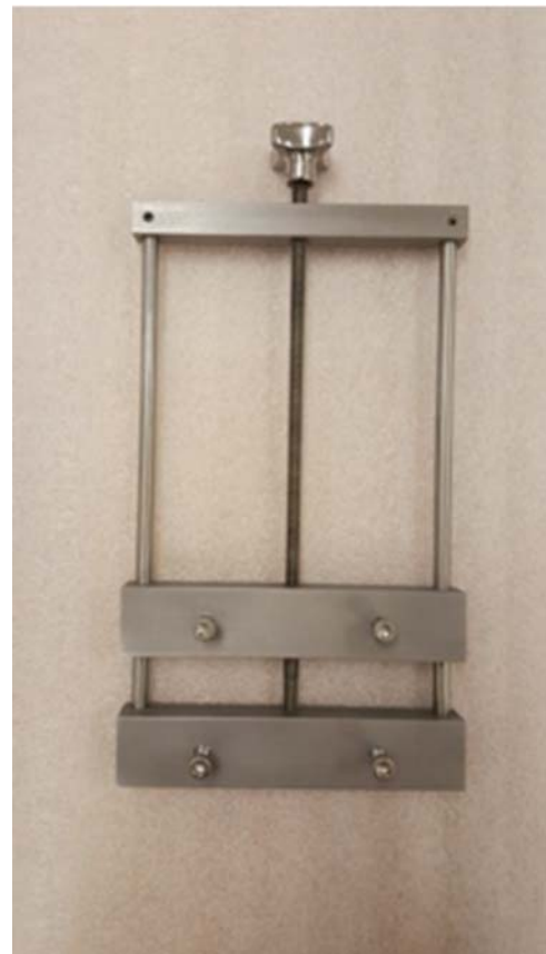
FIG. 5 Alternative Apparatus for Mounting Straight Rubber Test Specimens, Method B, Procedure B1
